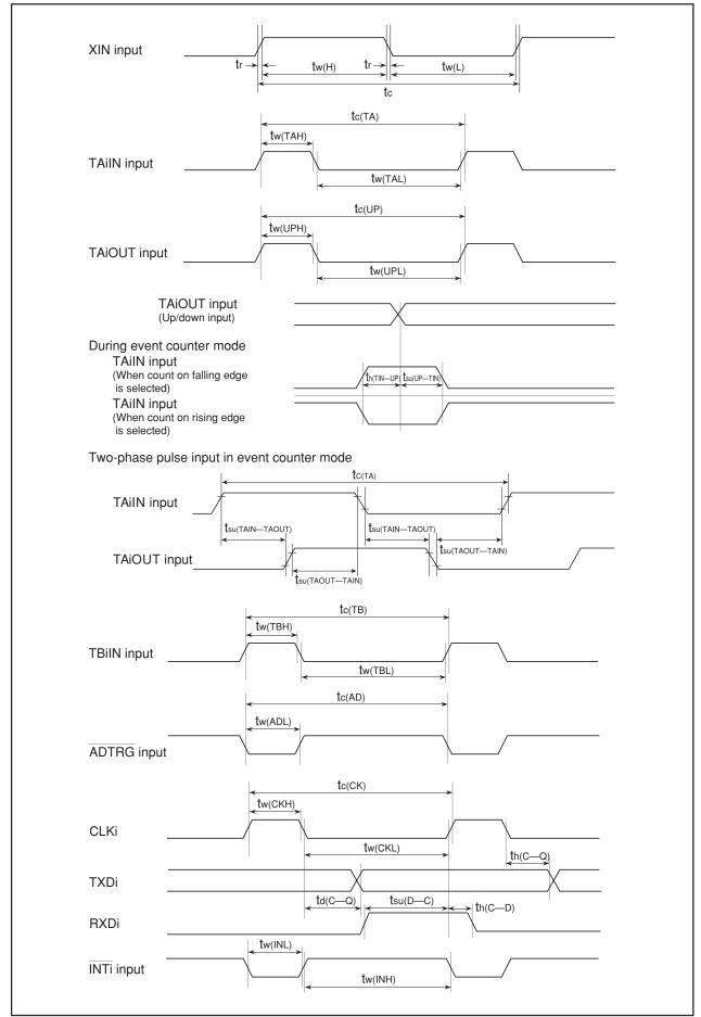
Figure 21.3 Timing Diagram
